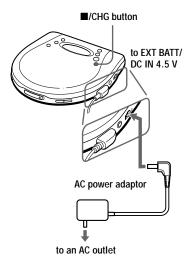
The CD player charges the batteries. The "CHG" indicator turns on in the display, and the indicator sections of \*\*TTL light up in succession. When the batteries are completely charged, the "CHG" and \*\*TTL indicators turn off.
